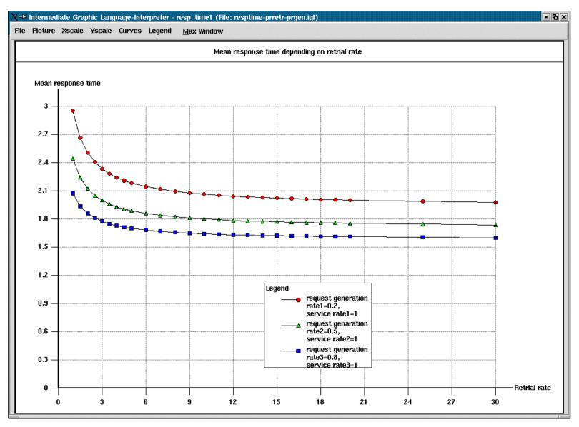
${\cal E}[T]$  versus retrial rate with homogeneous service and heterogeneous primary request generation
