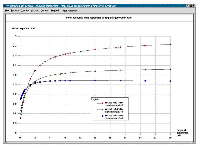
${\cal E}[T]$  versus primary request generation rate with heterogeneous service and heterogeneous retrial
