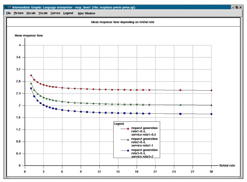
${\cal E}[T]$  versus retrial rate with homogeneous primary request generation and heterogeneous service
