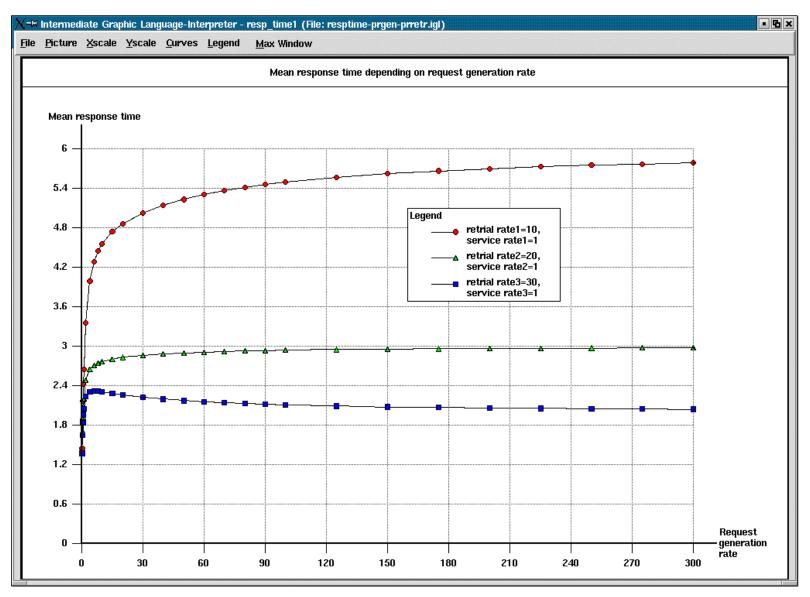
${\cal E}[T]$  versus primary request generation rate with homogeneous service and heterogeneous retrial
