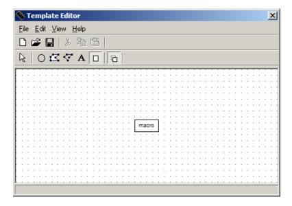
Now it is time to change the look of the macro to fit a MUX. It is possible to change and add shapes, text and pins. Pins are used to connect wires to the input and output of the macro. You can move text with move precision by using Ctrl + ArrowKey. Here is what you might end up with:
