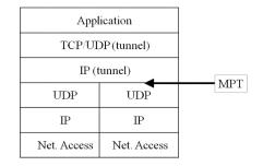
Fig. 1 The Layered structure of the MPT communication environment
