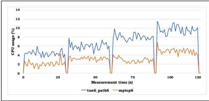
Figure 5: MPT-MPTCP CPU utilization comparison in a quad-path IPv6 Fast Ethernet multipath network environment in case of TCP Cubic and *iperf3*
