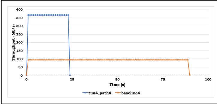
Figure 3: MPT-GRE IPv4-IPv4 *wget* throughput performance using 4 interfaces and the Cubic TCP congestion control algorithm
