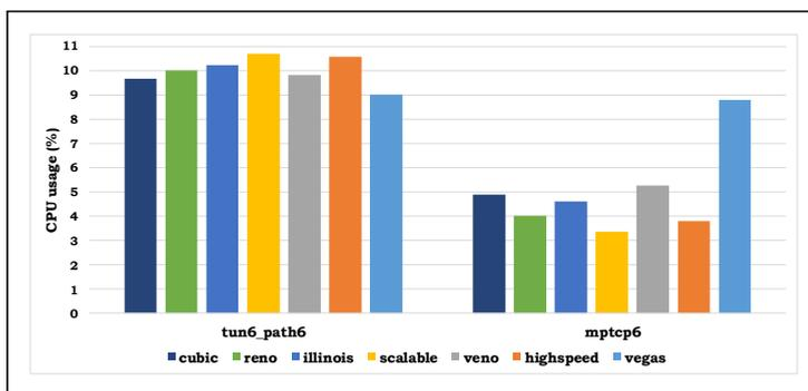
Figure 7: MPT-MPTCP CPU utilization comparison in a quad-path IPv6 Fast Ethernet multipath network environment in case of TCP Cubic, Reno, Illinois, Scalable, Veno, HighSpeed and Vegas using *iperf3*
