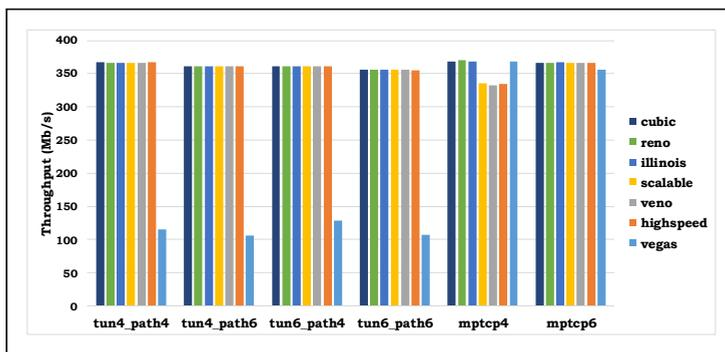
Figure 2: Testing the *iperf3* and FTP throughput performance of the MPT-GRE and MPTCP in quad-path IPv4/IPv6 Fast Ethernet environments
