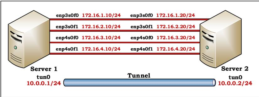
Figure 1: Quad-path Fast Ethernet measurement environment
