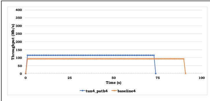
Figure 4: MPT-GRE IPv4-IPv4 *wget* throughput performance using 4 interfaces and the Vegas TCP congestion control algorithm
