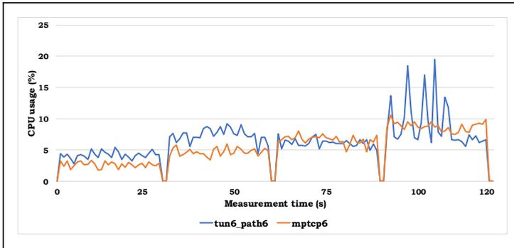
Figure 6: MPT-MPTCP CPU utilization comparison in a quad-path IPv6 Fast Ethernet multipath network environment in case of TCP Vegas and *iperf3*
